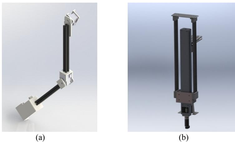
**Fig. 3.** Manipulator (a) and ball-screw drive system (b)
