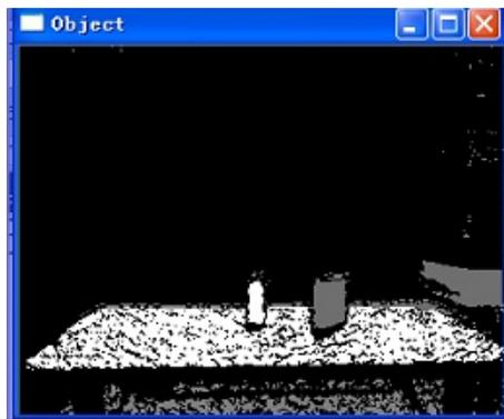
Fig. 8. The extracted table surface and graspable object
