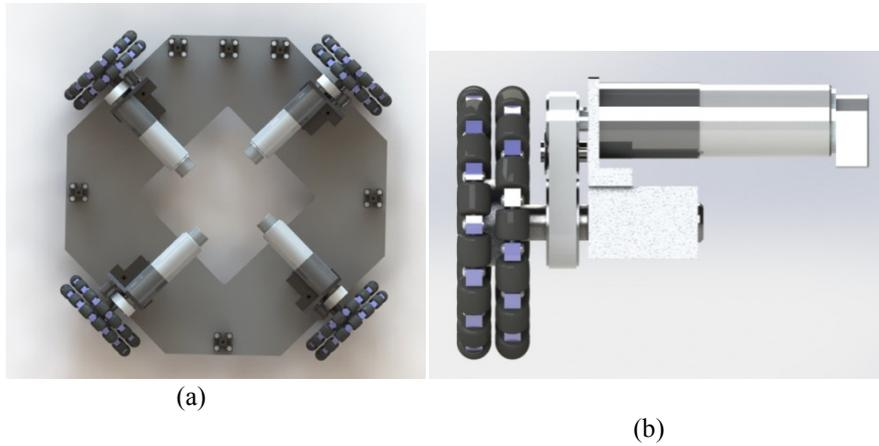
**Fig. 2.** Render of mobile base (a) and rendering of wheel mounting assembly (b)
