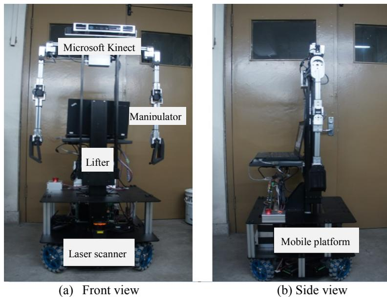
Fig. 1. Robot platform hardware
